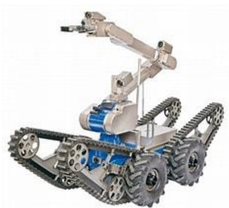
Obr. 9: Pyrotechnický robot Telex Explosive Ordnance Disposal Robot
